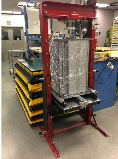
Figure 3-76. Stack Mechanically Loaded in Pre-compression Stand
