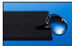
Water repelled by laser treated surface
