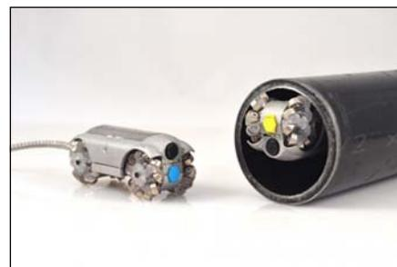
*Self-Propelled Pipe Crawler with Camera Attachment*
