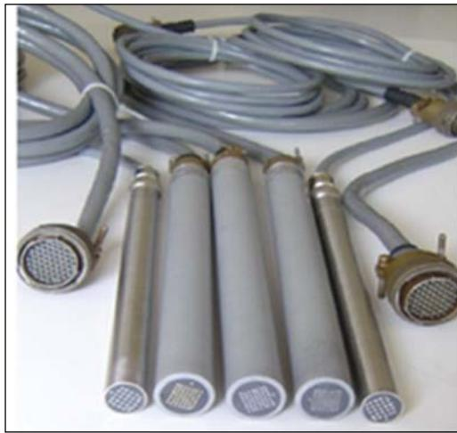
*NanoCorr Tank Corrosion Probes*
