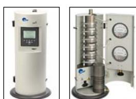
*Cascade Impactor with Multiple Impact Plates*
