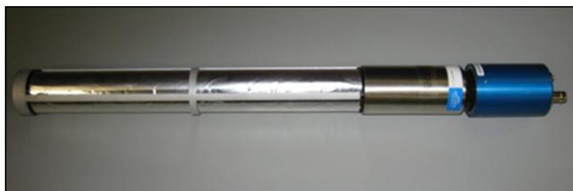
*Direct-Push Prototype Beta Detection Probe*
