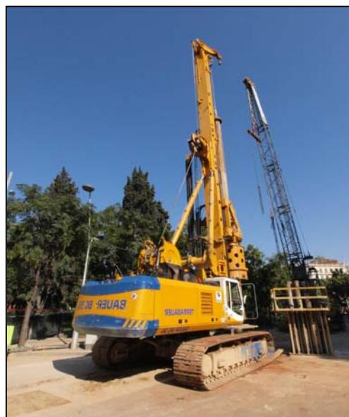
*Mobile Rotary Core Driller*
