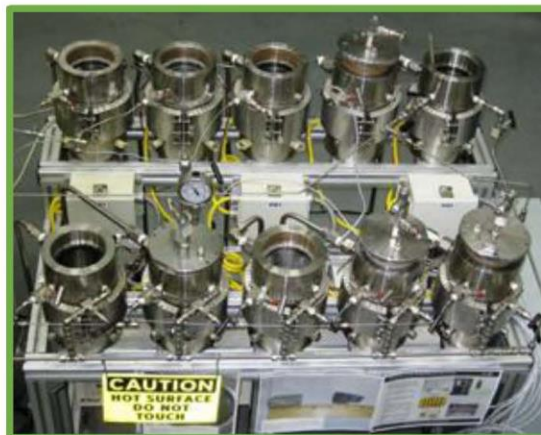
Static batch reactors for long-term experimentation
