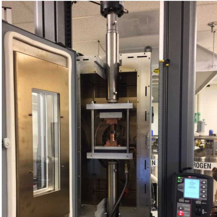
Experimental setup for evaluating motor material bulk and interface thermal resistance up to 200°C.
