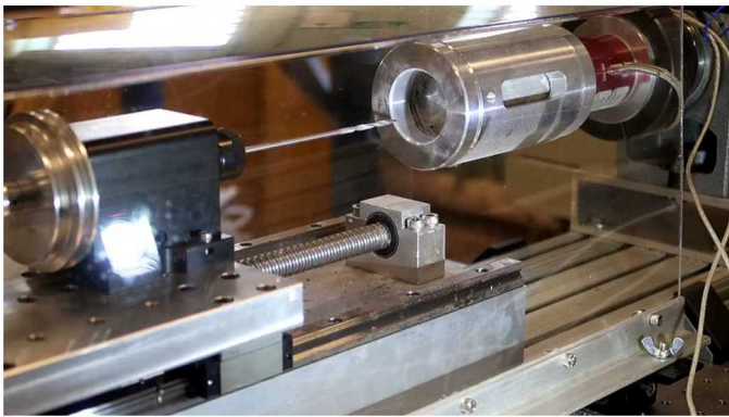
Fig. 2. Benchtop set-up designed to simulate microdrilling into wellbore casing.
