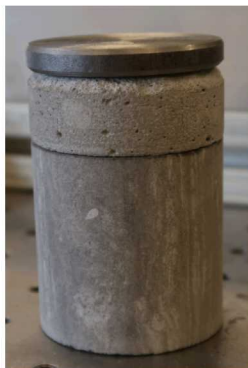
Fig. 3. Test sample material “sandwich” used for microdrilling with material in order of steel, cement, shale.
