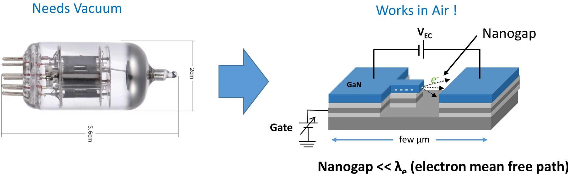
**Solid state “vacuum” nanoelectronics integrates advantages of vacuum devices and semiconductor nanofabrication**
