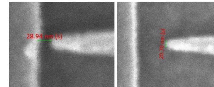
GaN structures down to ~30 nm gaps and ~20 nm wide emitters
