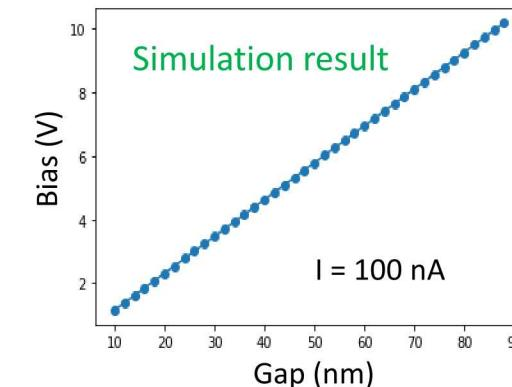
Bias voltage linearly depends on the gap size for fix field emission current
