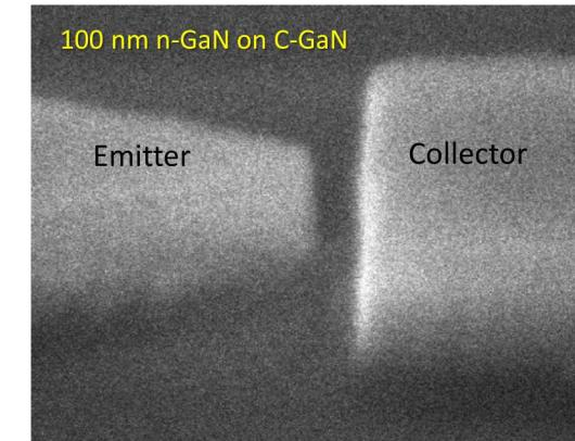
**ICP dry etch:** Angled side walls – variable gap size, possible shorting at bottom, sidewall damage
