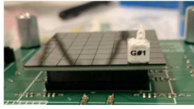
Fig. 2. (6\text{mm})^3 organic glass cube coupled to a SiPM array pixel.
