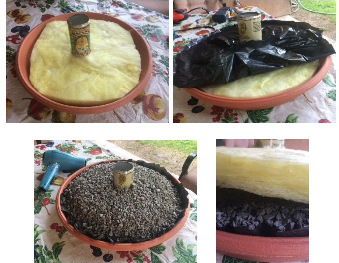
Figure 3. Sequence of photos showing the assembly of the bench-scale radial-thermocline test.
