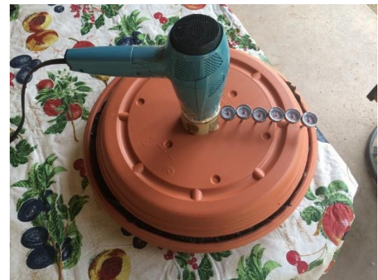
Figure 4. Assembled bench-scale test with thermometers and hair dryer in place.
