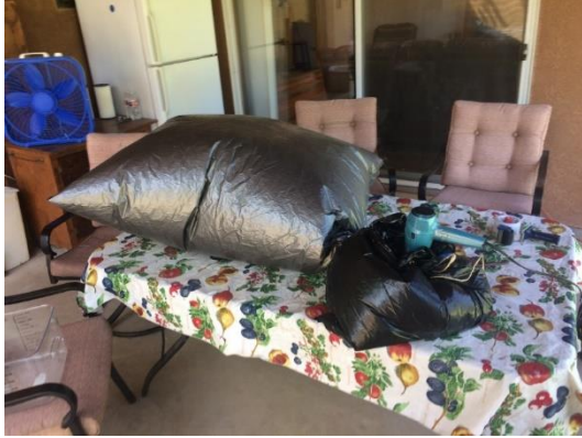
Figure 5. Measurement of airflow using a trash bag.
