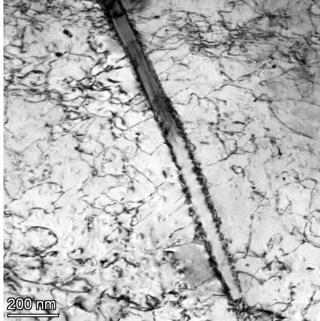
Figure 17. Creep deformation microstructure at 973 K (700°C), 325 MPa, Aged 263. \langle 200 \rangle g. An \eta plate (running almost vertically) appears to be a potent source of matrix dislocations, which are bowing out from the interface into the matrix. Note the fine ( \sim 30 nm diameter) \gamma' particles that precipitated during creep.
