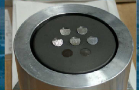
Angled DiMES specimens for testing at combined high-heat/particle flux
