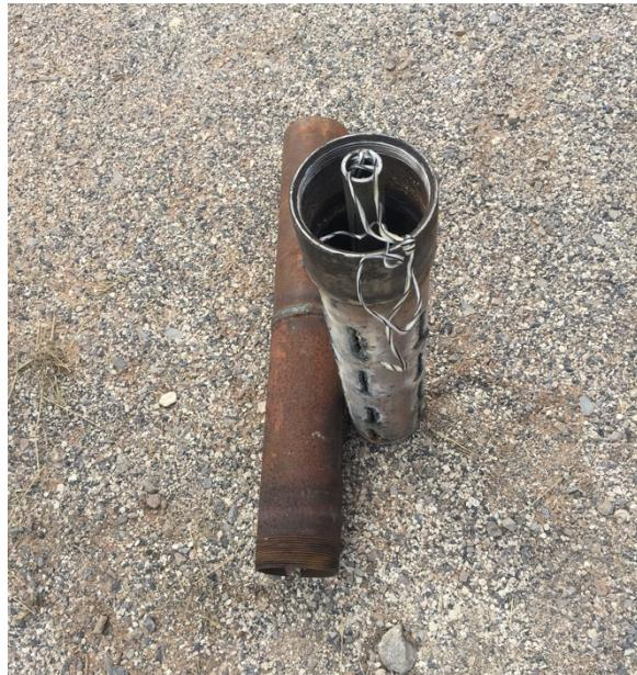
**Figure 6. Assembled sub with air slots above**
