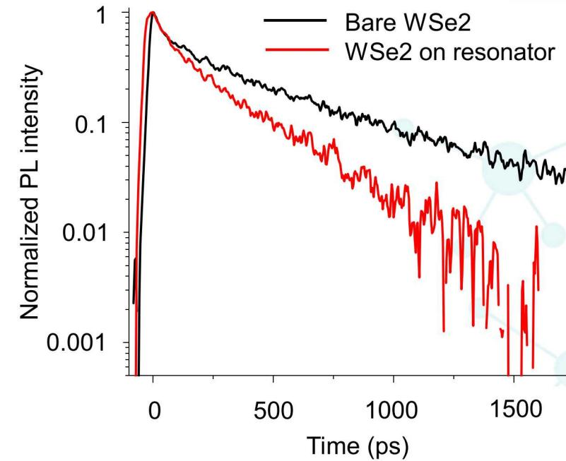
\* Toroidal metasurfaces can modify emission from 2-D materials placed atop via Purcell effect
