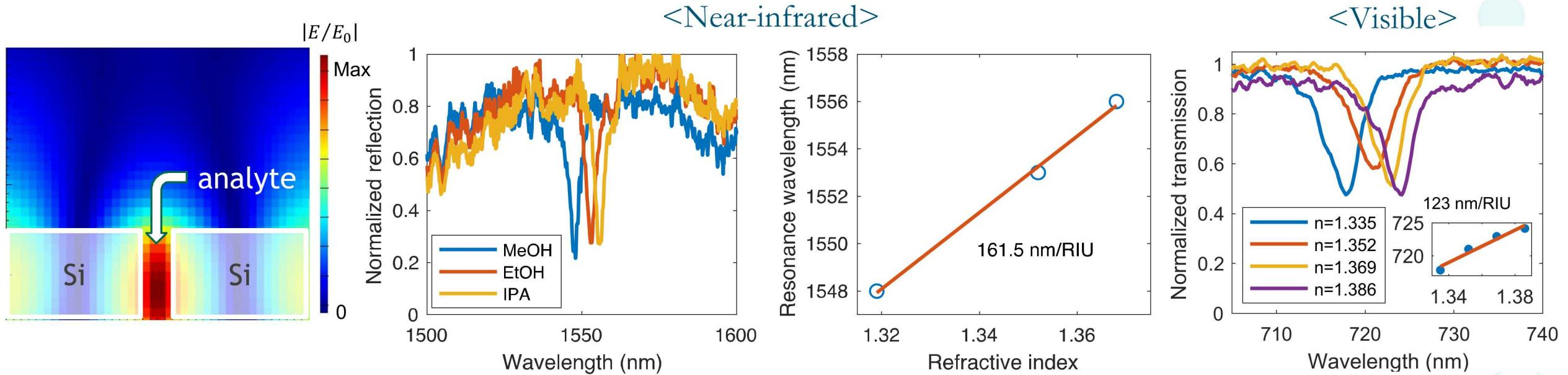
\* Strong field enhancement at the void allows efficient refractometric sensing
