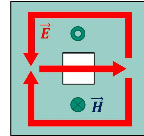
\* High-Q resonance with toroidal electric field profile is observed near 1500 nm
