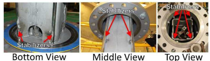
FIGURE 3: PHOTOGRAPHS OF THE TEST ASSEMBLY SHOWING THE BASKET STABILIZER RODS.
