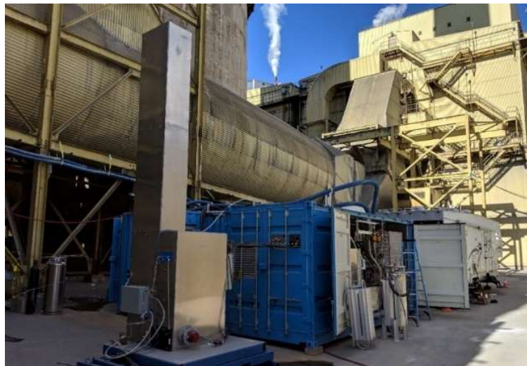
Figure. 3. CCC-ECL test skids at the PacifiCorp Hunter coal-fired power plant.
