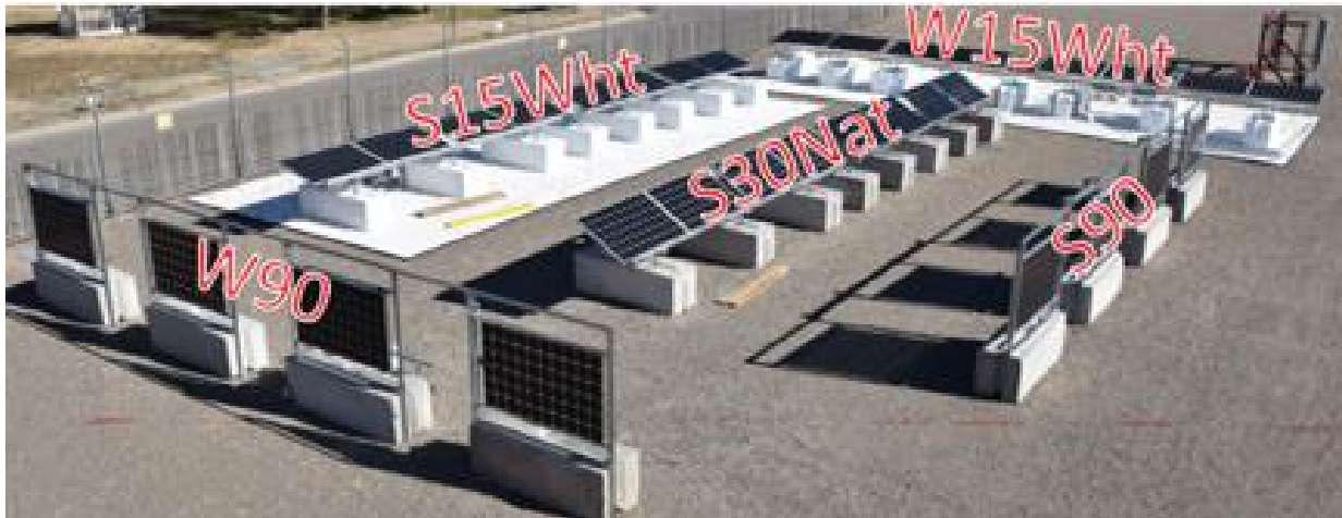
Figure 65: Prism Solar bifacial test array at Sandia National Laboratories in Albuquerque, New Mexico USA.
