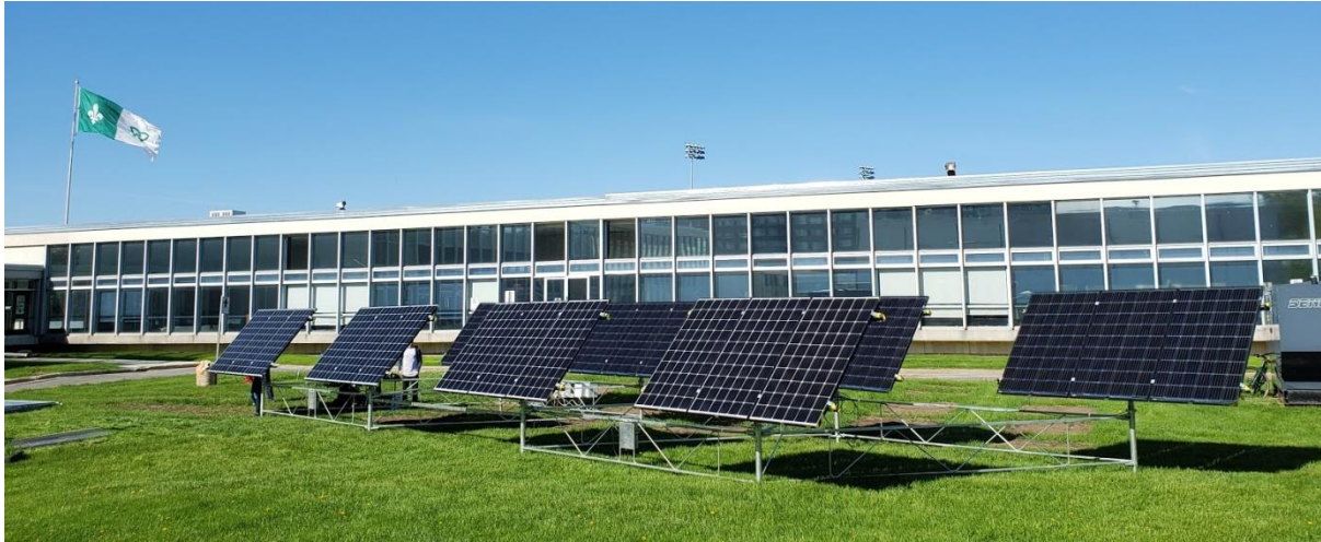
Figure 77: Two of three Savanna trackers installed at the University of Ottawa SUN-LAB field test site prior to the ASPIRE project
