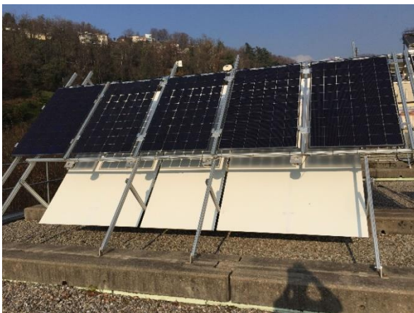
Figure 84: Bifacial test stand installed at SUPSI within the Swiss Project ENHANCE. (top row) Configuration including 3 monitored bifacial modules, 2 dummy modules, and 1 reference monofacial module in open-rack layout. (bottom row) Front view and side view, respectively, of white reflectors mounted behind bifacial PV modules.
