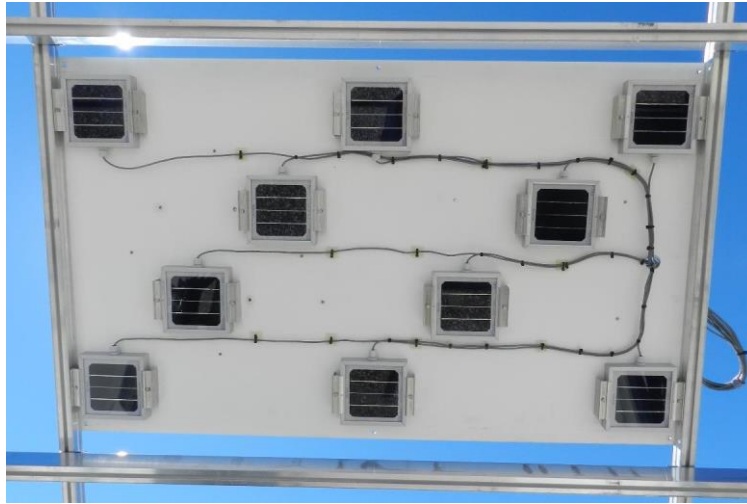
Figure 20: Rear view of the Sandia irradiance distribution module (IDM) showing the placement of the ten reference cells.
