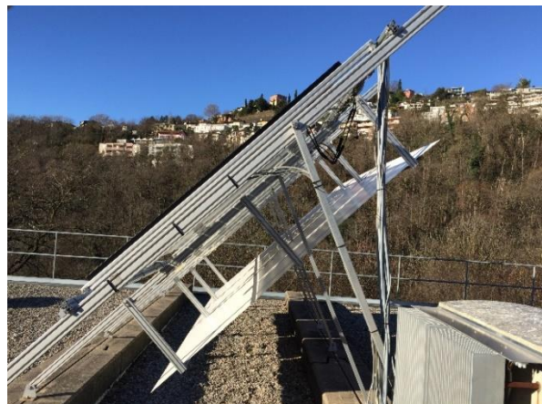
Figure 84: Bifacial test stand installed at SUPSI within the Swiss Project ENHANCE. (top row) Configuration including 3 monitored bifacial modules, 2 dummy modules, and 1 reference monofacial module in open-rack layout. (bottom row) Front view and side view, respectively, of white reflectors mounted behind bifacial PV modules.
