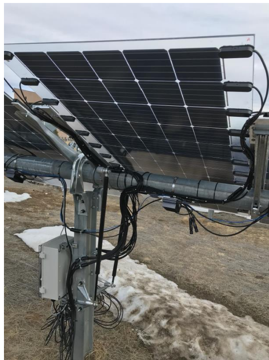
Figure 91: Custom module with 12 individually addressable strings mounted in the middle of NREL's bifacial PV field
