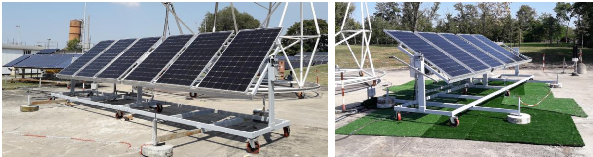
Figure 107: Bifacial PV system under test; South-facing PV module on light grey concrete tilted 30°(left); South-facing PV modules on synthetic green grass tilted 30° (right).
