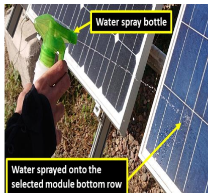
Figure 1-29: Soiling - Water sprayed
