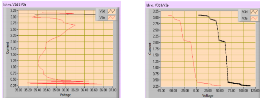
Figure 2-21: IV curve result comparing direct (black) and non-contact (red) measurements
