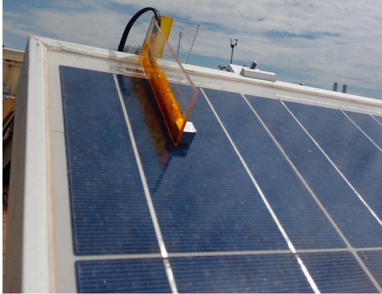
Figure 1-9: Probe (Trek 344) with Probe Holder
