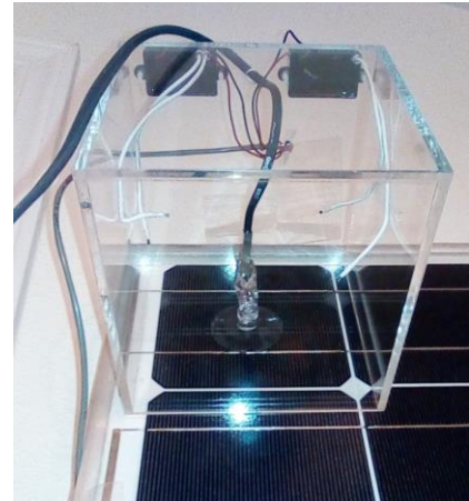
Figure 2-27: Miniature air ionizers inside mini-environment
