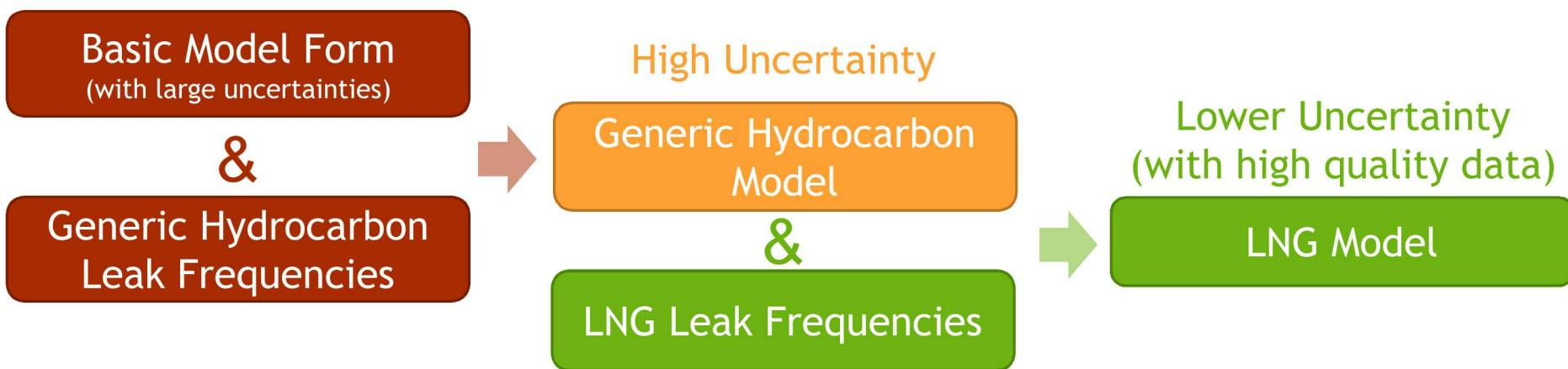
Model can be readily updated with liquid hydrogen leak data provided by industry partners to improve the estimated leak frequencies
