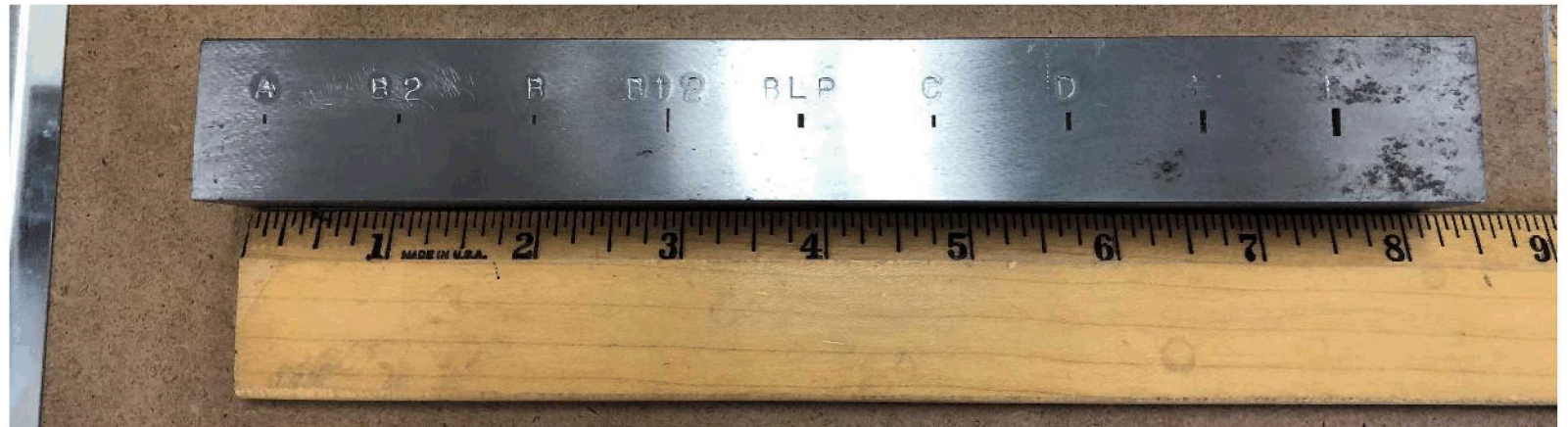
Calibration block with machined defects
