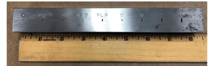
Calibration block of manufactured defects
