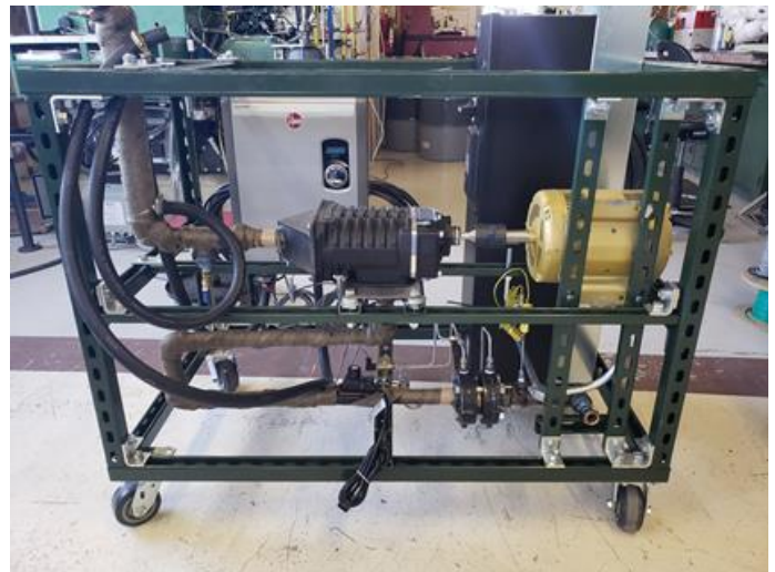
Figure 2: Custom Exhaust Gas Recirculation Test Cart for CFR Engine.
