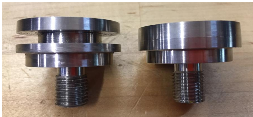
Figure 2: Left: Photo of creviced RCM piston used in homogenous ignition delay experiments Right: non-creviced pistons used for flame speed and F-egai experiments.
