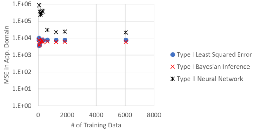
Figure 3.15: MSE of Dittus-Boelter correlation and machine-learning-based closure in the application domain.
