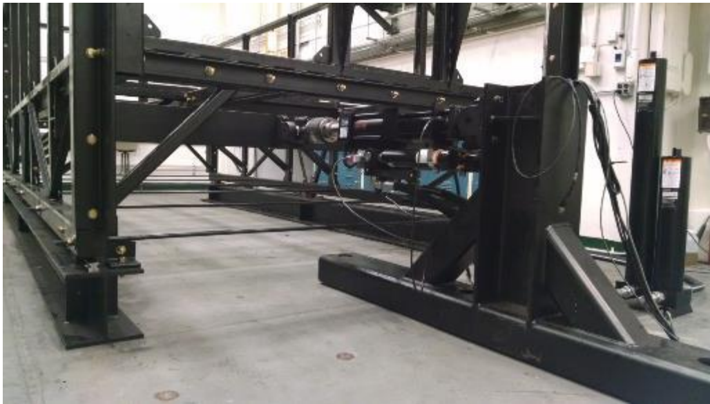
Figure 7.28. Actuator connected to the tank and strong floor support.
