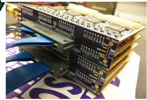
Full 64/128 channel electronics module (Custom IRS3D ASICs)
