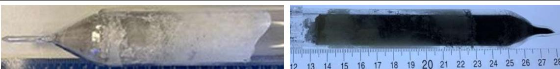
Fig. 1. The results of the two-stage purification process for (a)  $\text{Cs}_2\text{HfCl}_6$  (CHC) and (b)  $\text{Ti}_2\text{HfCl}_6$  (THC).
