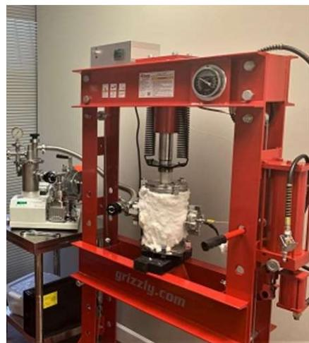
Fig. 3. One of the pressing setups at XI, Inc. consisting of 20-tons capacity presses with portable controlled heating chambers connected to a vacuum pump.
