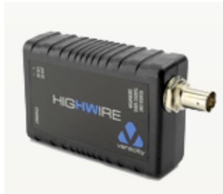
Figure 3. Commercial Ethernet over coax cable adapter. (source https://www.veracityglobal.com/media/59081/highwire_vhw-hw200-150.png )
