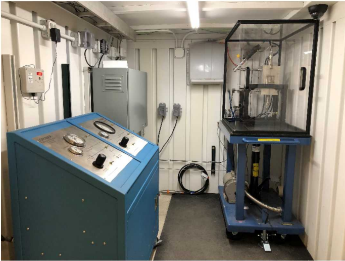
FIGURE 2: Pressure Vessel Test Rig in secondary containment with pressure cart on front left, electrical enclosure rear left, and test stand and H2PC™ on right
