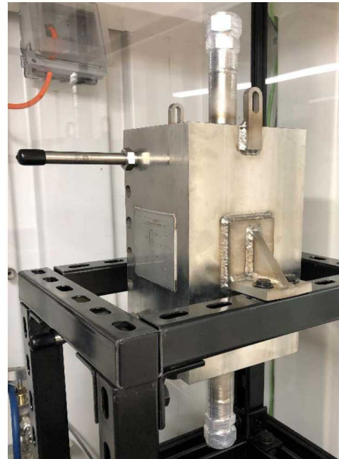
FIGURE 1: Hydrogen Pre-cooler under test.
