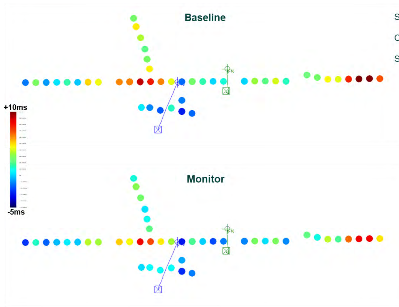
Figure 8-24. Statics - Plane view with statics for each SP. Static shift values were calculated separately for the baseline and the monitor survey.
