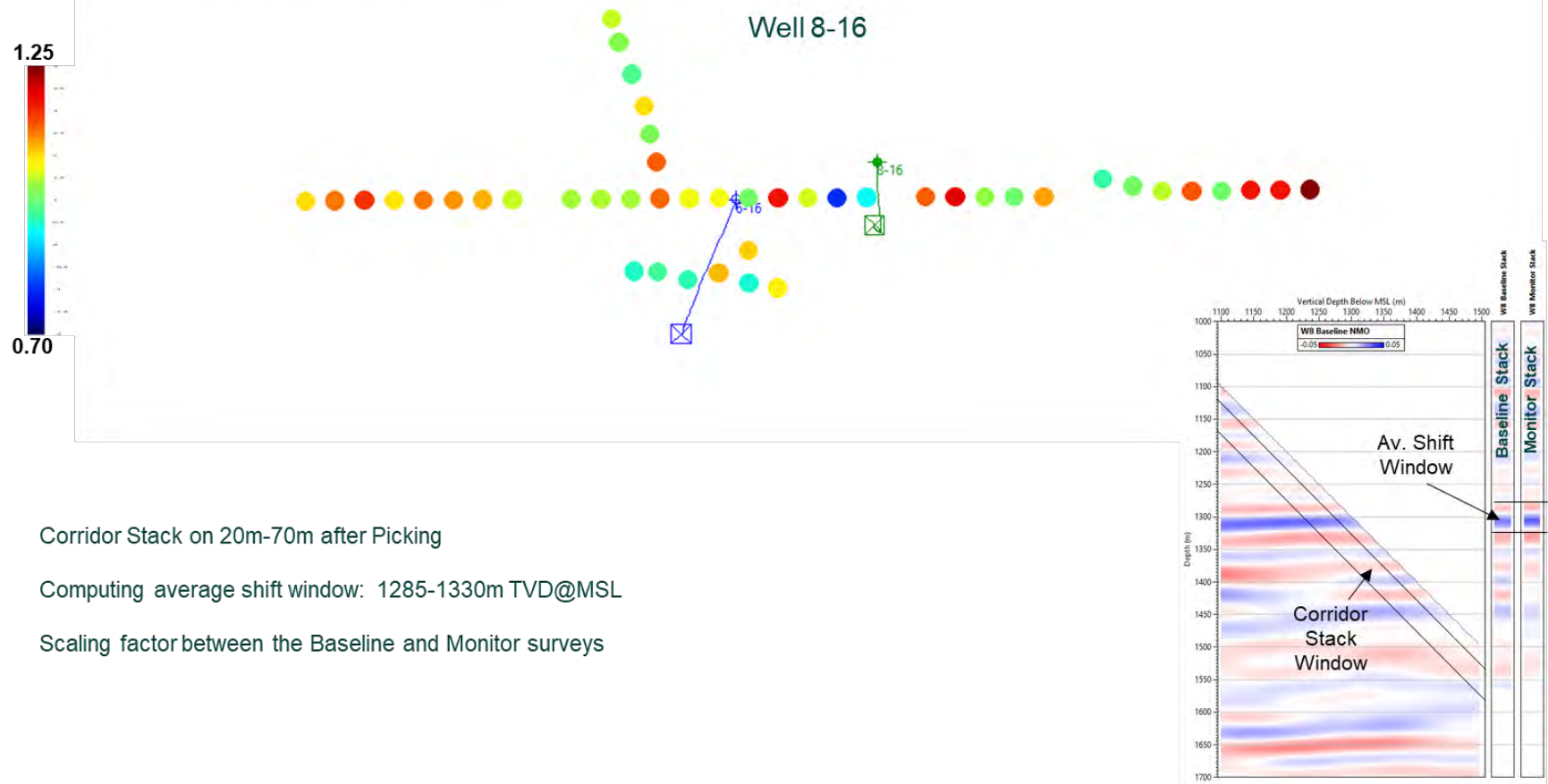
Figure 11-20. Monitor Scaling factor– Well 8-16 - For each SP. For well 8-16 data the scaling factor was computed using the RMS values extracted from the baseline and monitor NMO corridor stacks over the 1285 m to 1330 m TVDMSL interval (Fig. 11.20 right).
