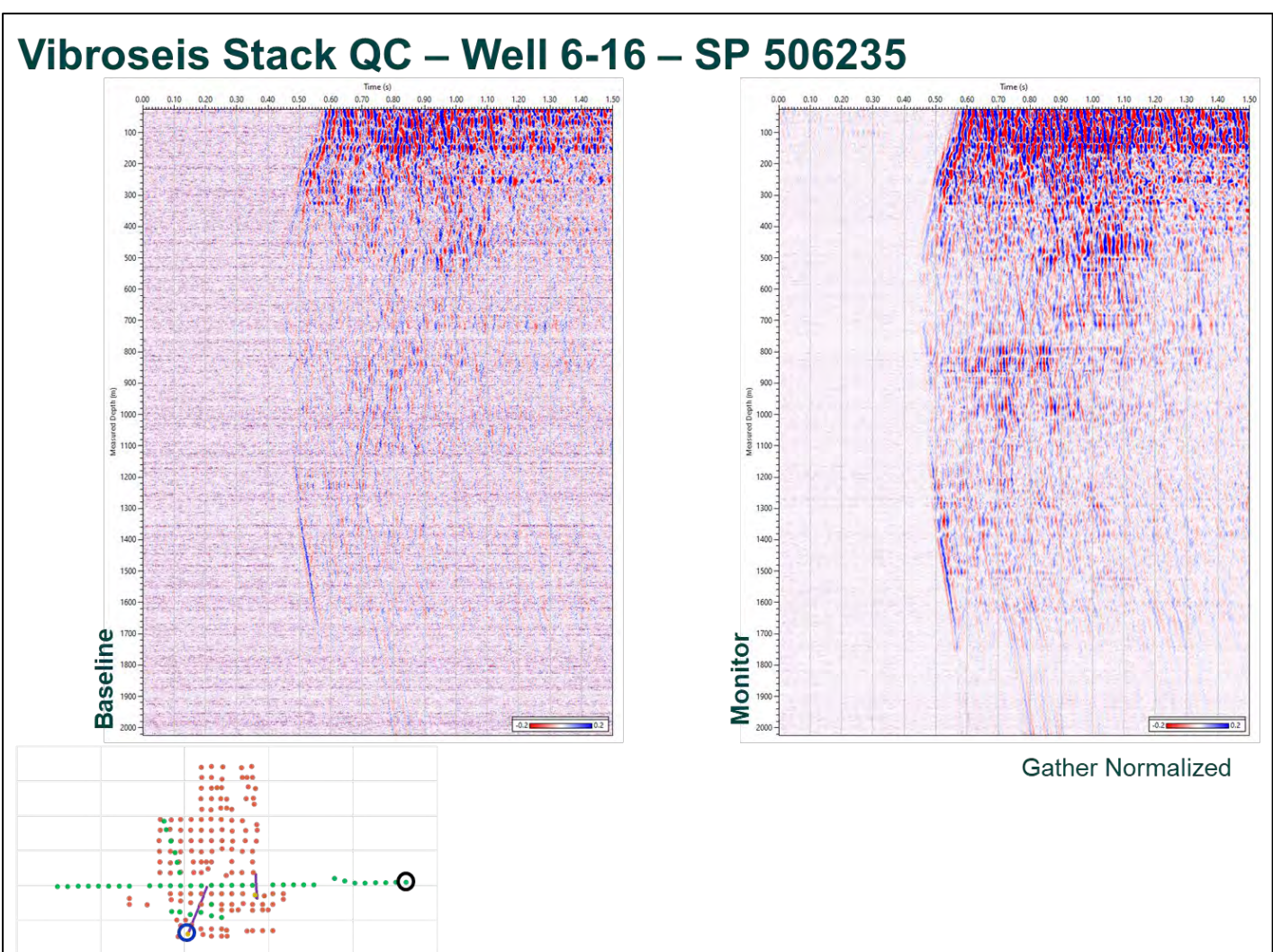
Figure 6-40. Vibroseis Stack QC – Well 6-16 – SP 506235 - Baseline and monitor survey.
