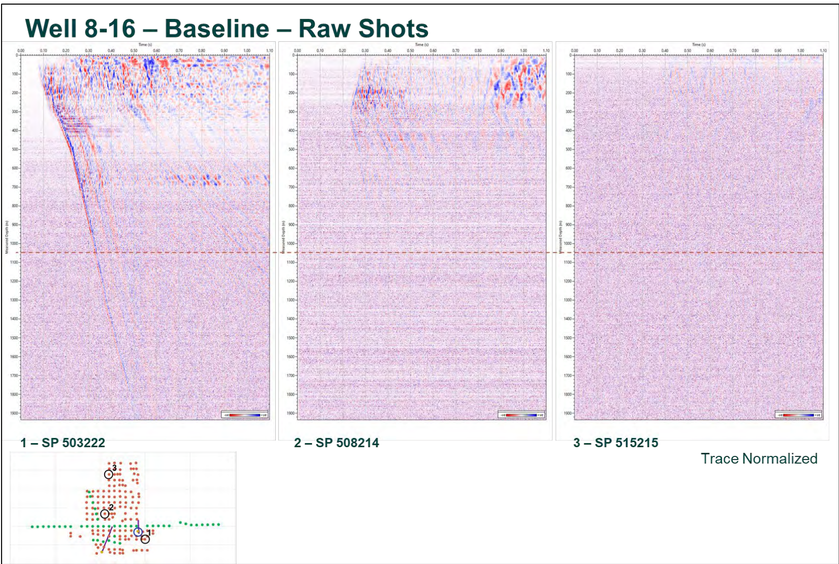
Figure 9-3. Well 8-16 – Baseline – Raw Stacks - Far, mid and near offset total wavefield.
