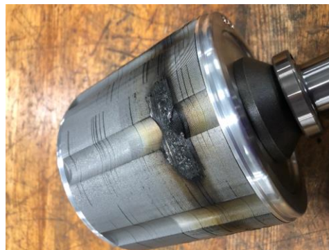
Figure 17: Variant 2 rotor after rotor endurance failure.
