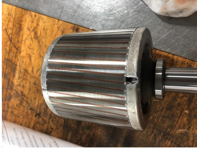
Figure 17: Variant 3 rotor after rotor endurance failure
