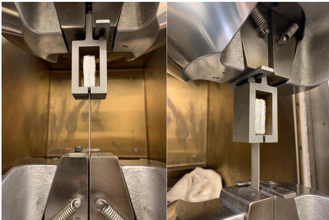
Figure 24: Custom test fixture made for testing rotor bars
