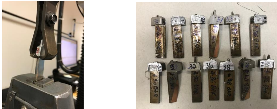
Figure 9: Rotor test coupons and test setup from casting development
