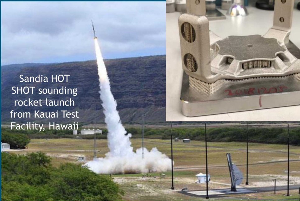
316L SS HOT SHOT top cap on plate
