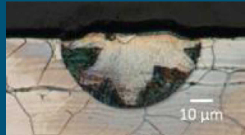
melt pool on plate, 100W, 1500 mm/s
