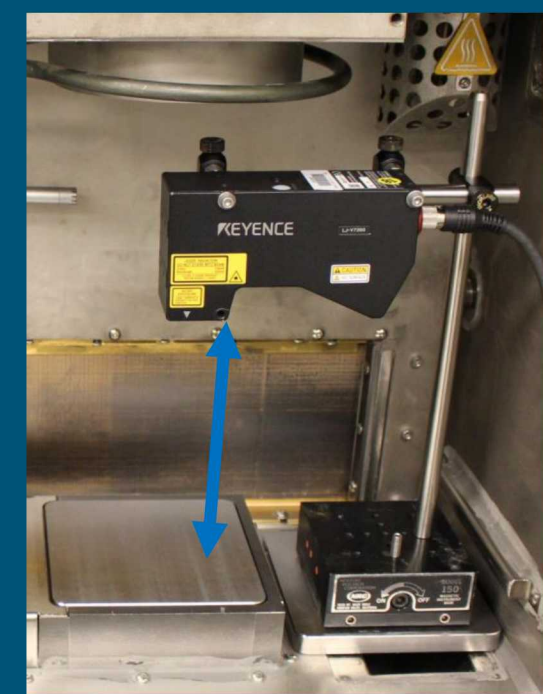
Keyence LJ-V7200 focused onto build plate
