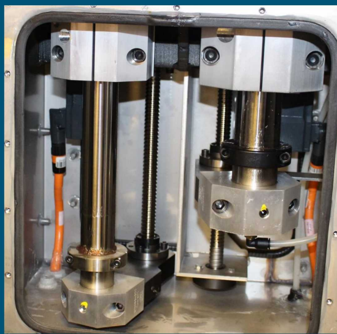
supply piston drive (left) & build piston drive (right)
