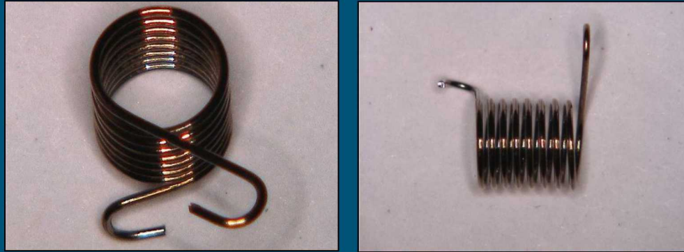
A representative meso-scale torsion spring. The wire diameter is 0.175mm, the spring length is 3.8mm, the coil diameter is 2.5mm, and the wire material is Elgiloy.
