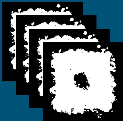
aligned & segmented bitmap stack white = material, black = air/void
