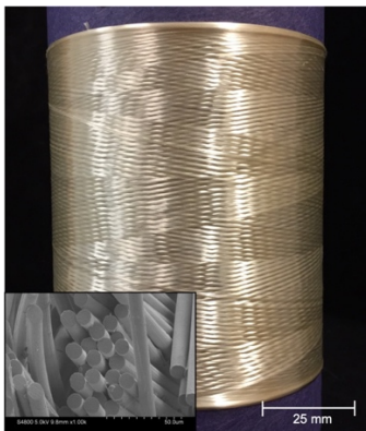
Figure 1. Typical spool of multifilament continuous TechPAN precursor fibers, with round, 10 \mu\text{m} fiber cross sections shown in the inset. A typical spool contained 1 km of multifilament tow length.
