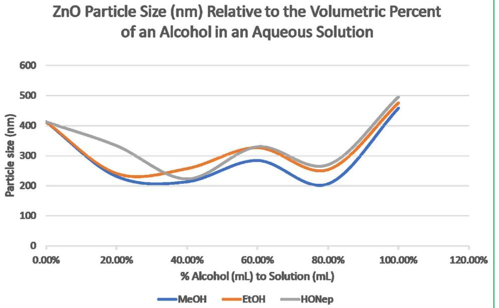
A plot of the size versus the concentration of alcohol shows the tunability of the final  $ZnO$ .
