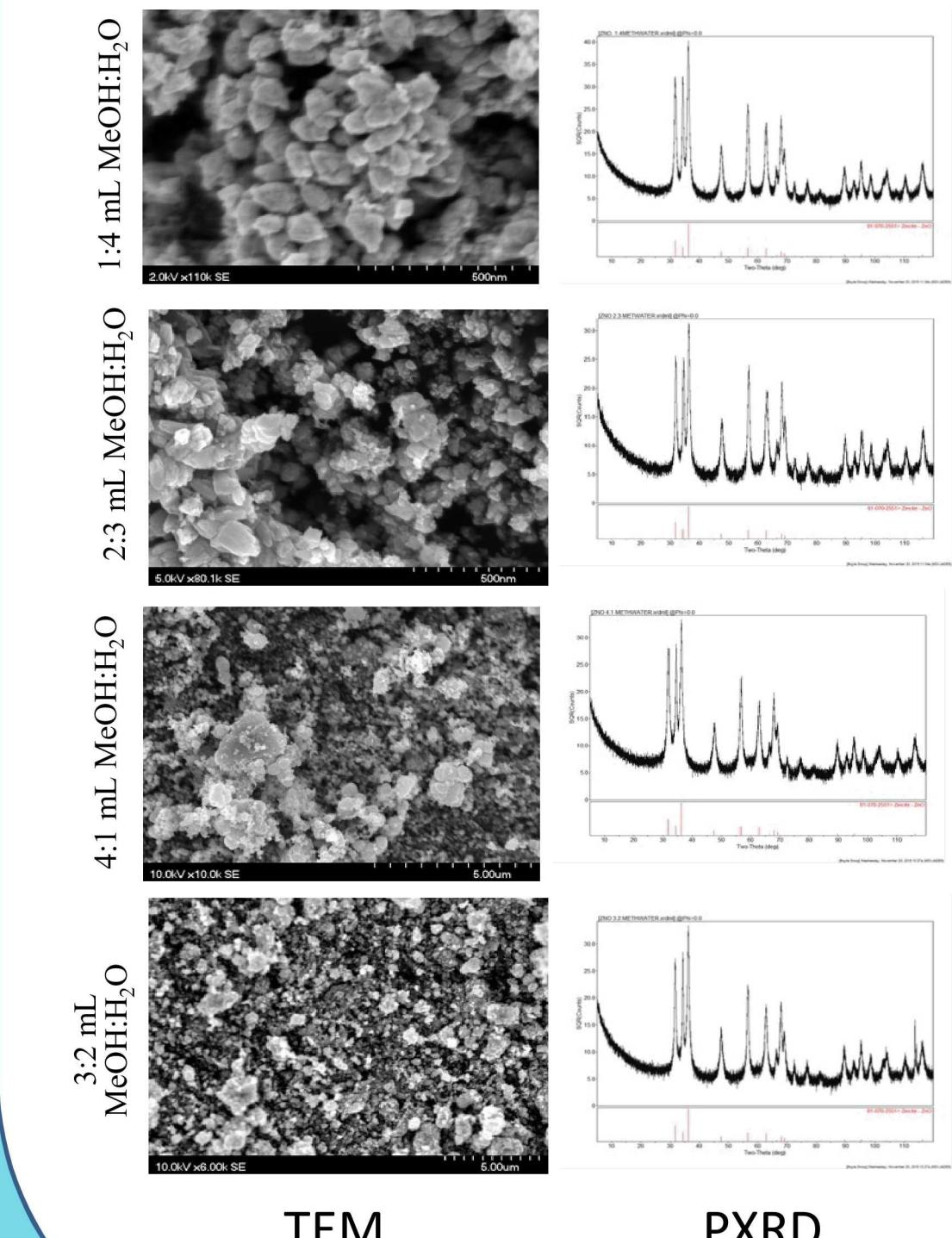
PXRD patterns verify the zincite phase had formed for each sample. TEM and DLS analyses indicated that the size of the particles could be controlled by the ratio of water and alcohol.
