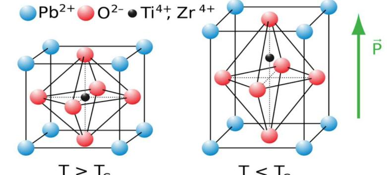
**Properties**: high dielectric constant; high coupling; high charge sensitivity; high density with a fine grain structure; a high Curie point; and a clean, noise-free frequency response, high piezoelectric charge constant; high mechanical quality reduces mechanical loss, lower operating temperature; low dissipation factor that ensures cooler, more economical operation; high dielectric stability; and low mechanical loss under demanding conditions
