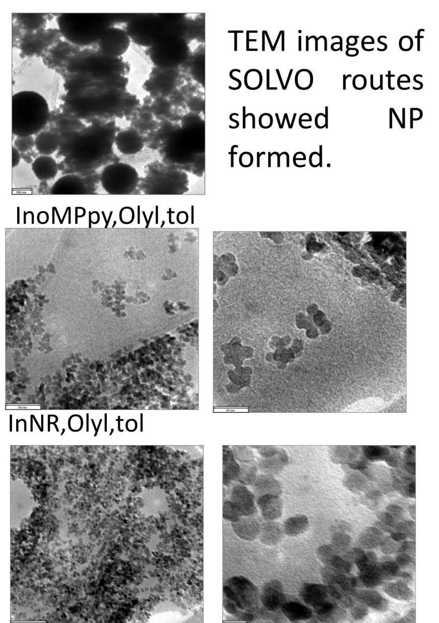
ITO solutions of varied stoichiometries were generated by mixing the two amide in toluene and processing under standard conditions.
