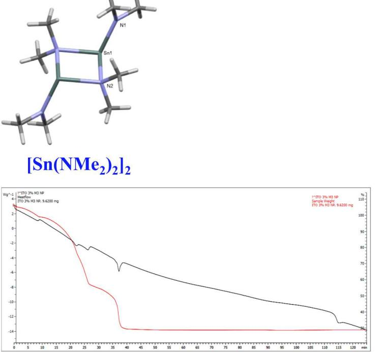
TGA/DSC data revealed decomposition of resulting ITO powder occurred below 250 °C.
