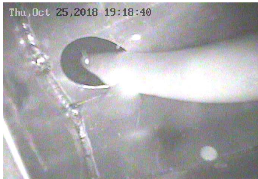
Figure 3-4. Video image of an eel entering the peripheral entrance of the horizontal bypass.
