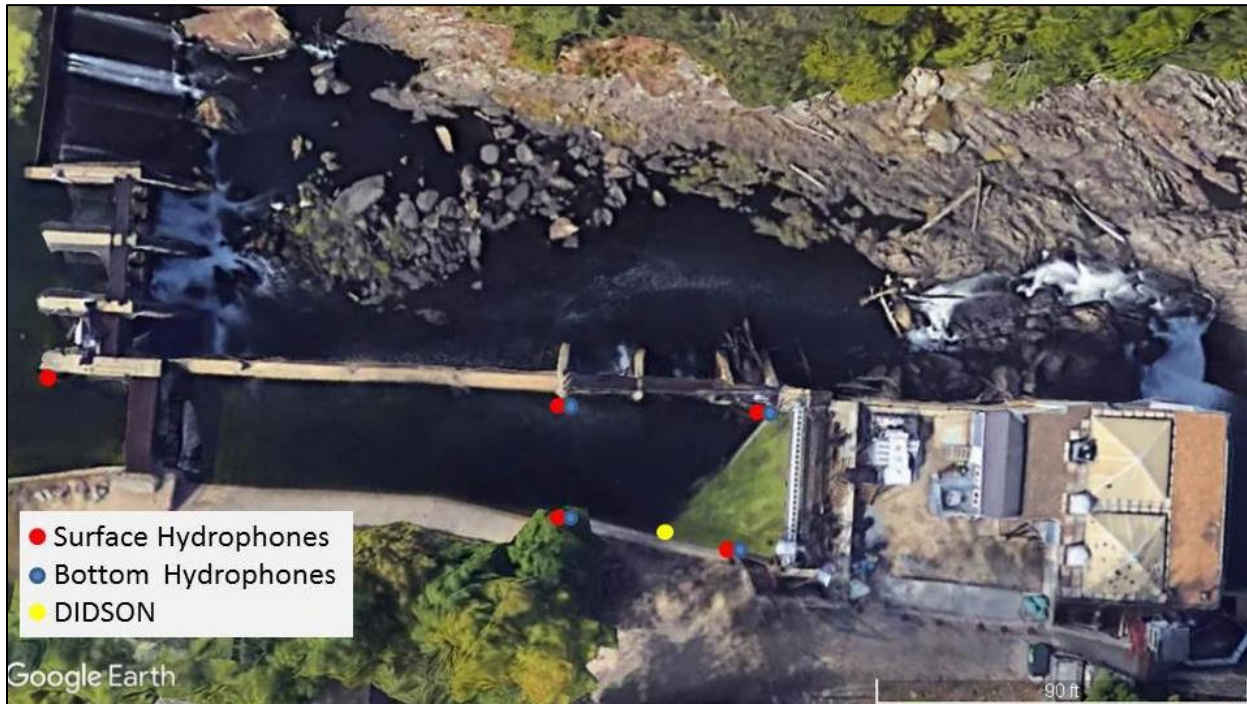
Figure 4-7. Location of acoustic hydrophones and DIDSON installed at the Mine Falls Project.
