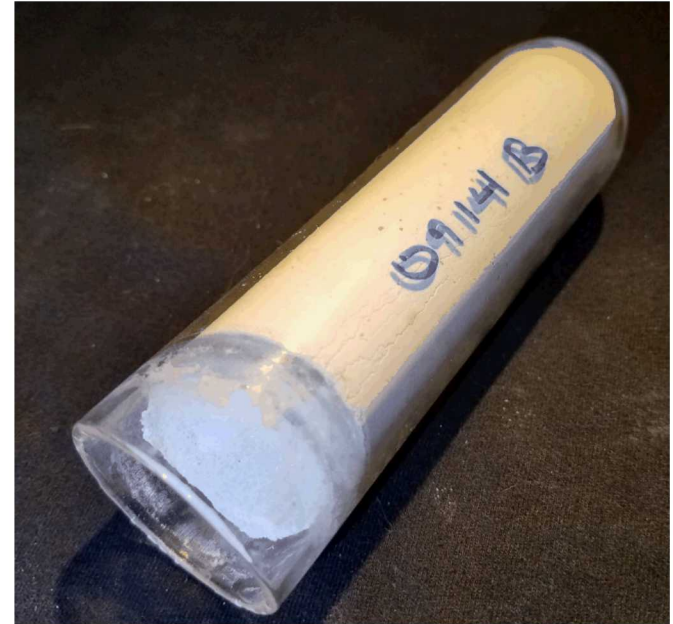
APC sample in Pyrex tube (1.25 in x 5 in) after setting and curing.
