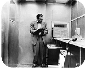
Laminar Flow Clean Room
