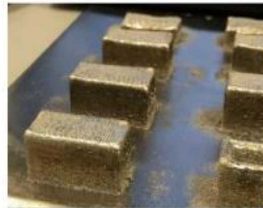
304L SS / Cu multi-material thermal concentrator
