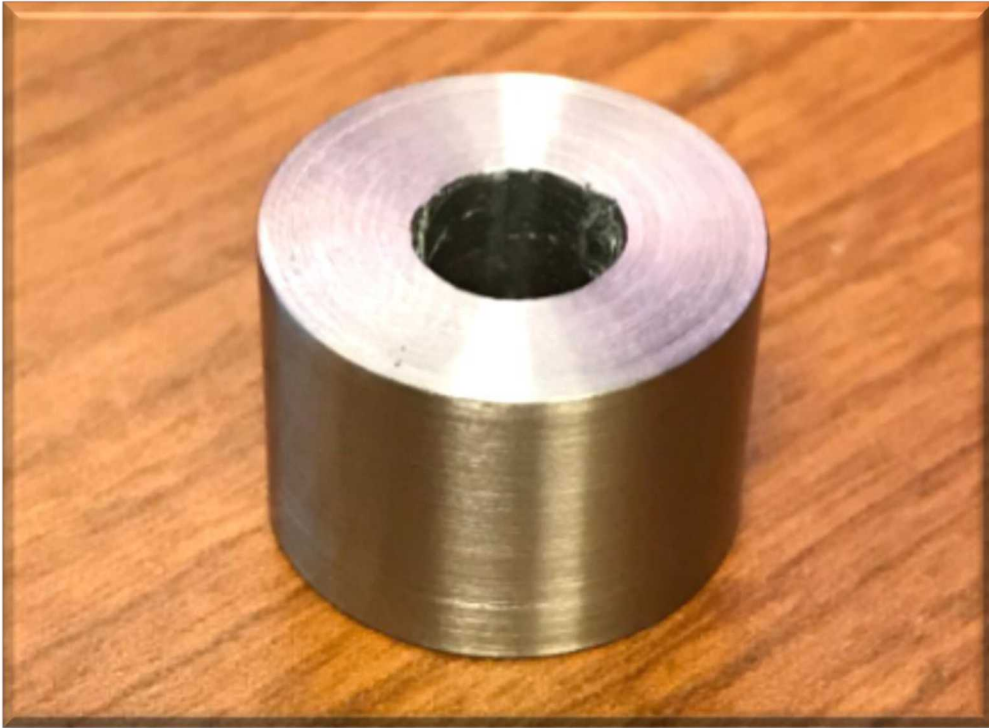
Multi-material and Hybrid Hiperco core with SS304L Shell
