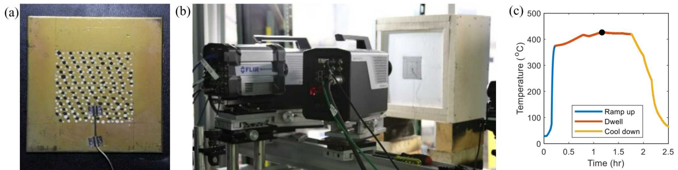
Figure 1: (a) Stainless steel test specimen, 3.5 x 3.5 inches (89 x 89 mm), with phosphor and black high-temperature paint features and a welded K-type thermocouple, after heating to approximately 400°C for 2 hours. (b) Overview of the test setup, showing two Shimadzu HPV-X2 ultra high-speed visible-light cameras, one FLIR S8300 mid-wave IR camera, and the test piece mounted in a vertically-oriented radiant heater. (c) Thermal history of one test, as measured by the specimen thermocouple. The black circle indicates one time step that is explored in later figures and analysis.
