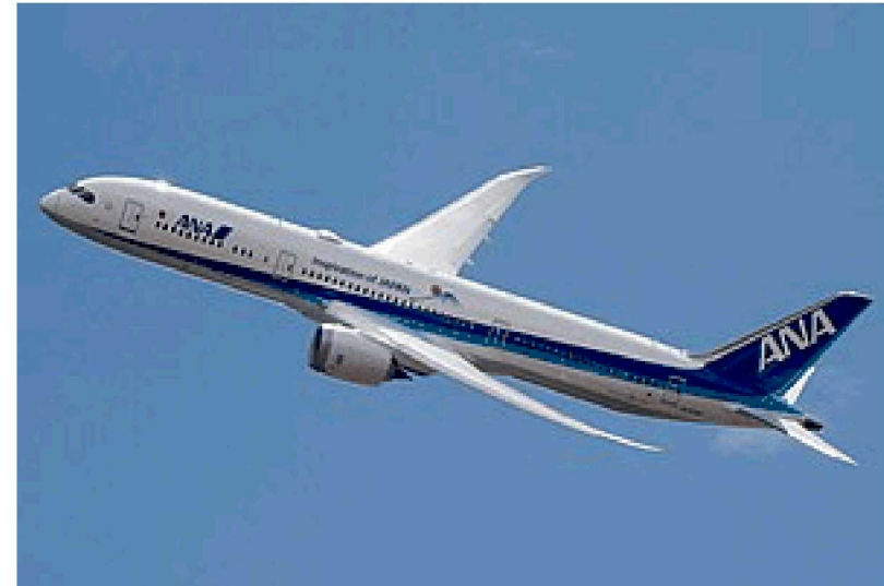
Boeing 787 Dreamliner airframe is 50% Carbon fiber epoxy composites
