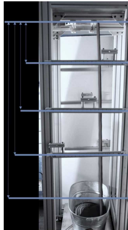
FIGURE 3: Baseline particle curtain: top hopper slot is indicated by the top line and light meter positions are indicated by the bottom four lines
