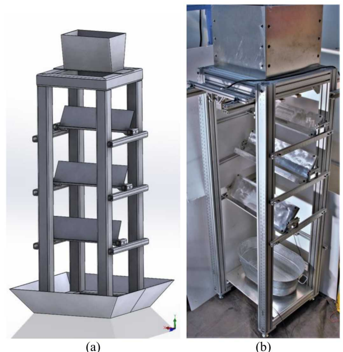
FIGURE 1: Particle flow test apparatus (a) conceptual design and (b) fabricated rig
