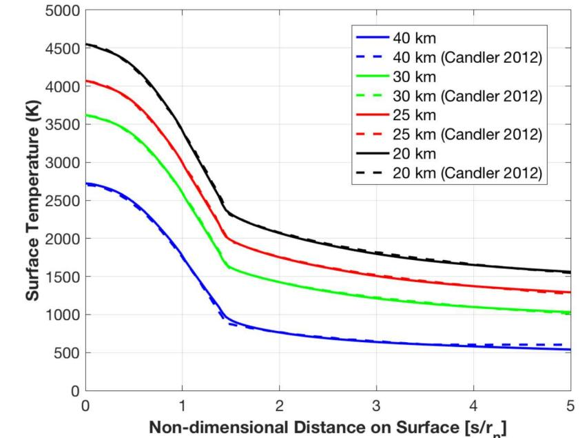
Surface temperature comparison between model and Candler's results for freestream speed of 7 km/s. Temperature profile serves as boundary condition for finite-rate models. Results found by using a non-catalytic non-ablating radiative equilibrium surface BC and run with Trajectory-US3D. Geometry in both cases was a 10 cm radius sphere - 8 degree cone geometry. All cases run with laminar boundary layer.
