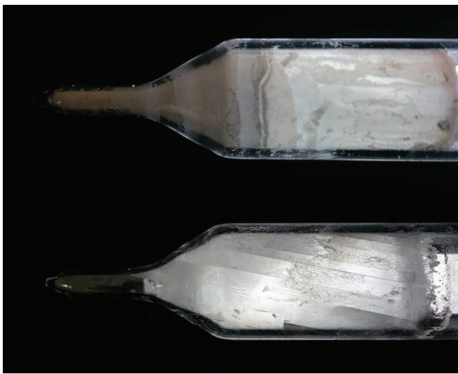
Figure 2. Photographs of \text{Tl}_3\text{GdCl}_6:\text{Ce}^{3+} (top) and \text{TlGd}_2\text{Cl}_7:\text{Ce}^{3+} (bottom) crystals grown at RMD.
