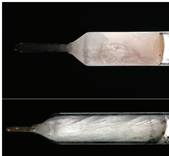
Figure 1. Photographs of \text{Tl}_3\text{YCl}_6:\text{Ce}^{3+} (top) and \text{TlY}_2\text{Cl}_7:\text{Ce}^{3+} (bottom) crystals grown at RMD.
