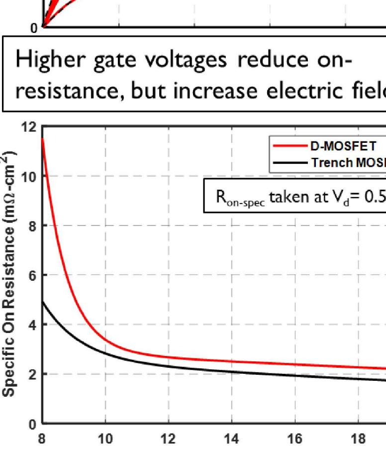
Higher gate voltages reduce on-resistance, but increase electric field
