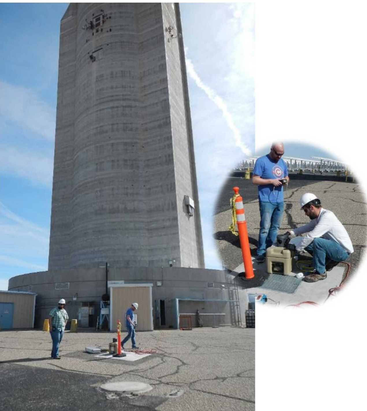
Above: Volumetric air sampling of small (<10 µm) particles during on-sun particle-receiver test
