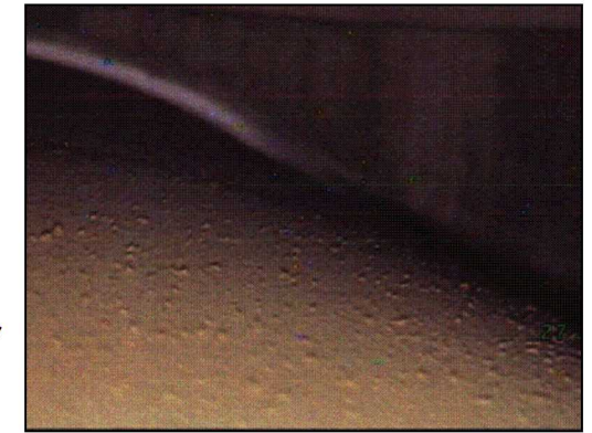
Dust on storage canister surface at Calvert Cliffs (EPRI 2014)
