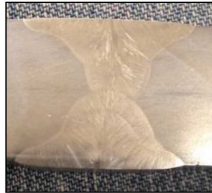
Weld zone, Ranor 304 SS plate
