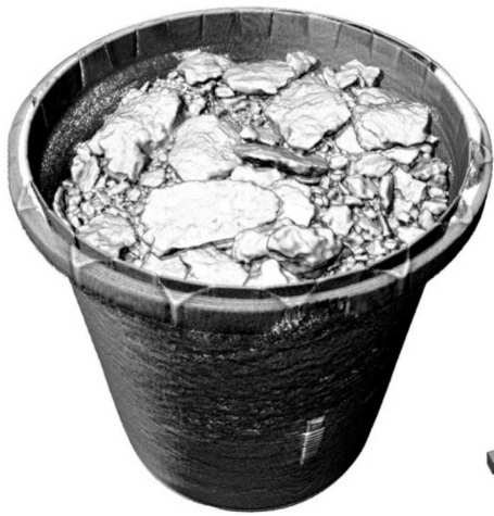
Figure 3. X-ray tomographic reconstruction of bucket of run-of-mine salt. The bucket is approximately 12" across.
