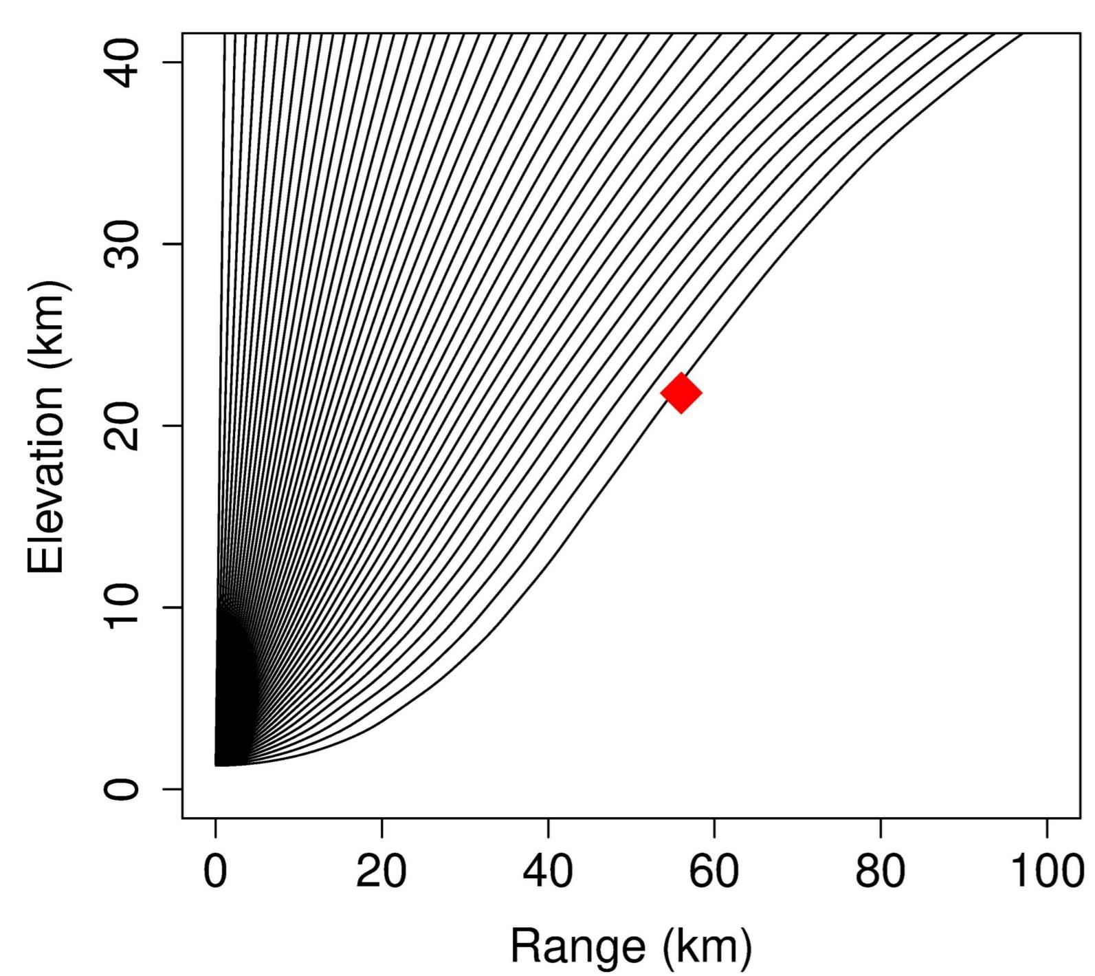
Acoustic ray paths from the DAG site towards the balloon-borne microbarometer. The red diamond shows the balloon's position when the acoustic signal was detected. The microbarometer was very nearly in the "acoustic shadow", a region in which no arrivals are expected. This effect is due to the upward-refracting characteristics of the lower atmosphere.
