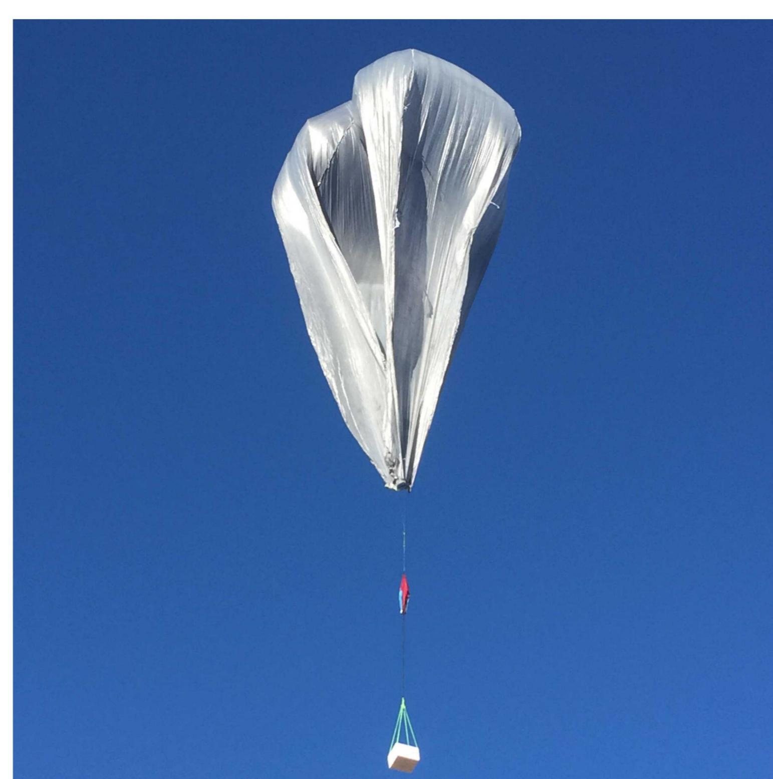
Acoustic waves were recorded on a Gem microbarometer on board a Heliotrope solar hot air balloon similar to the one shown above.
