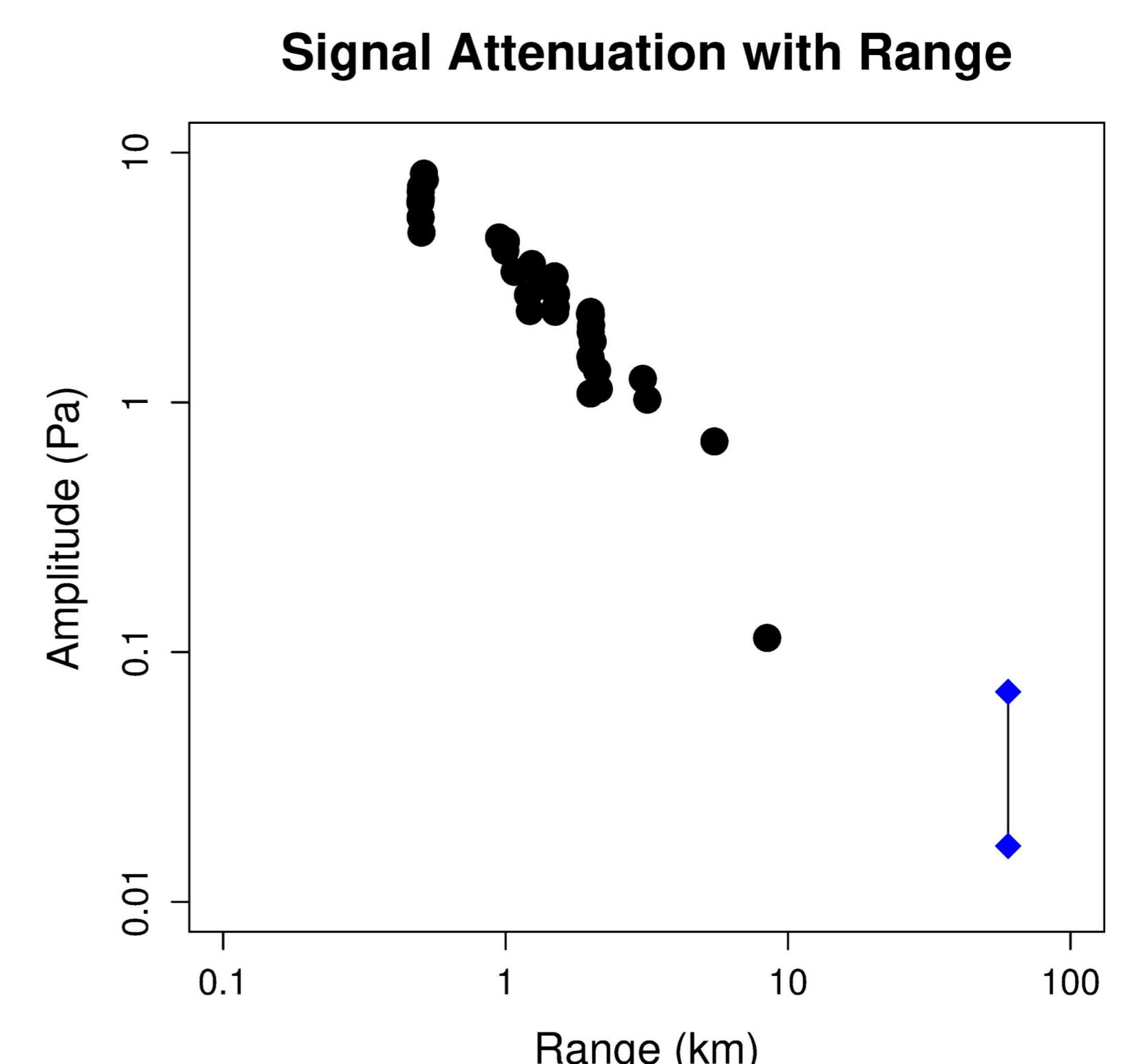
Signal amplitude compared to range for ground stations (black dots) and the balloon (blue diamond). The two balloon symbols show amplitudes adjusted and not adjusted for impedance contrasts.
