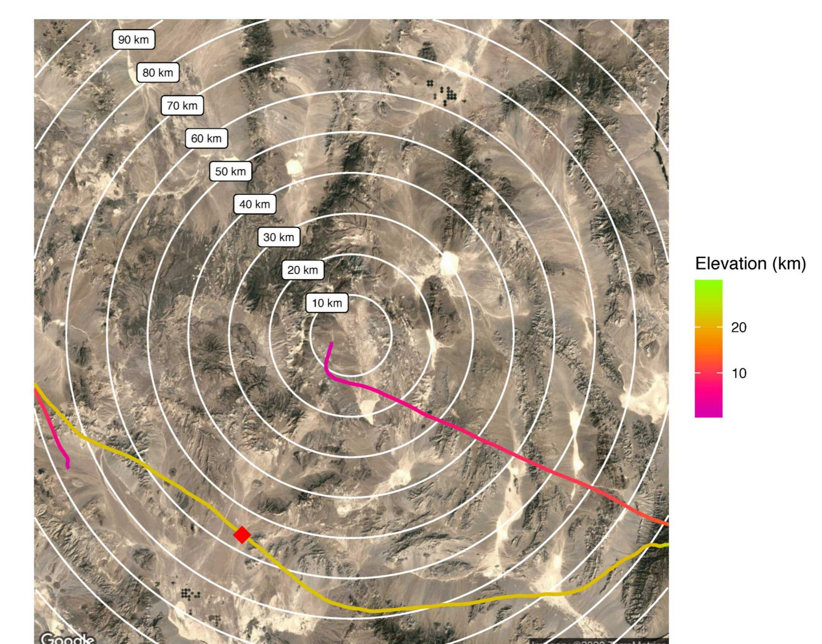
The trajectory of the balloon-borne microbarometer from its launch point 5 km west of the DAG site to its landing point in the Amargosa Valley. The red diamond shows the balloon's position when the DAG-4 signal was detected.
