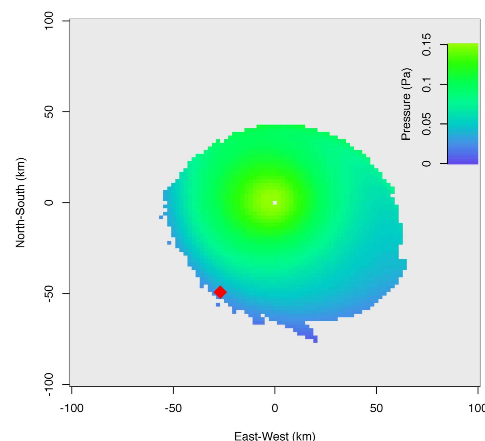
Expected pressure amplitudes at the balloon's elevation assuming an isotropically radiating source with similar overpressures as those recorded on the DAG-4 ground microbarometers (4 Pa at a range of 1 km). The plot takes both geometric and intrinsic attenuation into account, as well as amplitude reduction due to impedance contrast (approximately a factor of 4).
