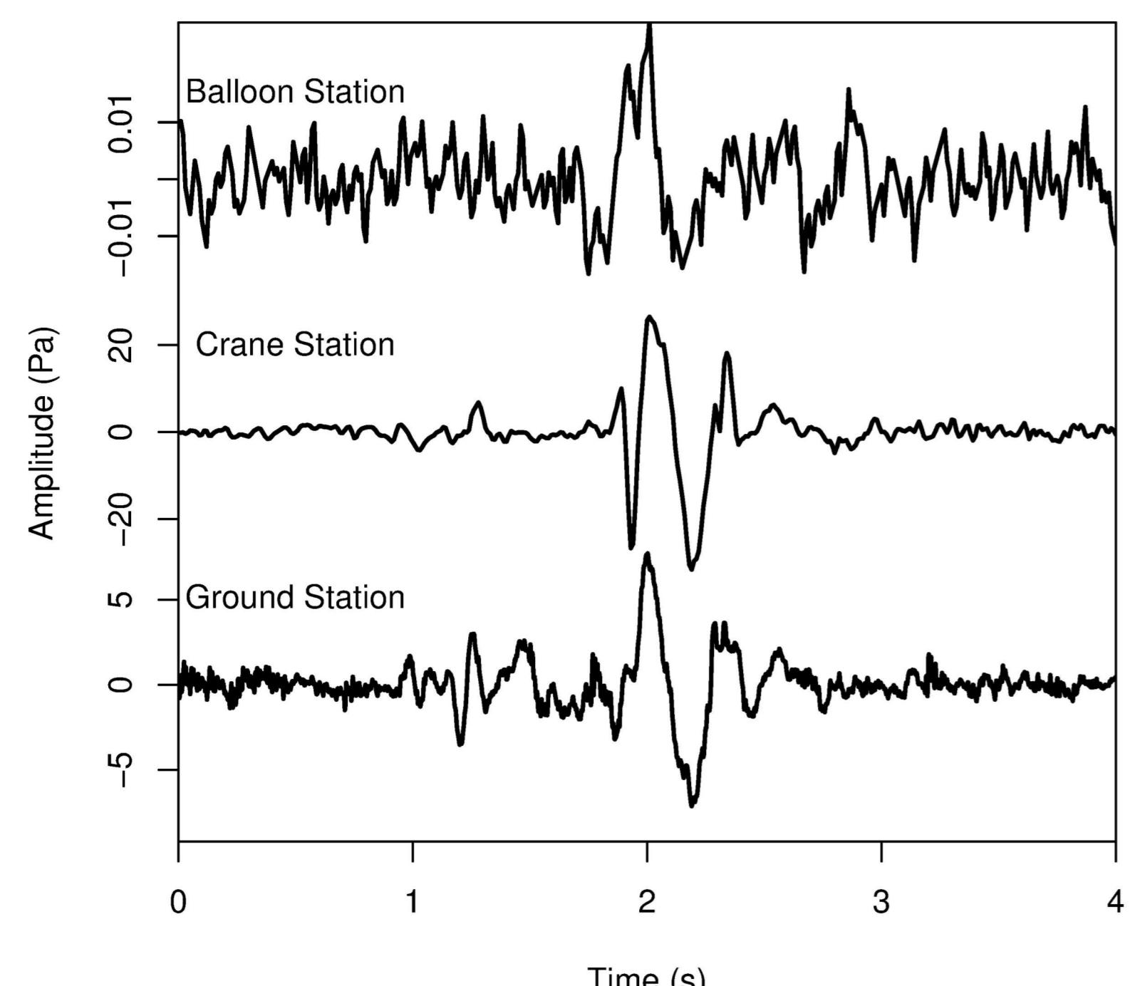
Waveforms recorded on the balloon (top) compared with those recorded atop a crane 34 m above the ground and 150 m from ground zero (middle) and a ground station 500 m from ground zero (bottom).
