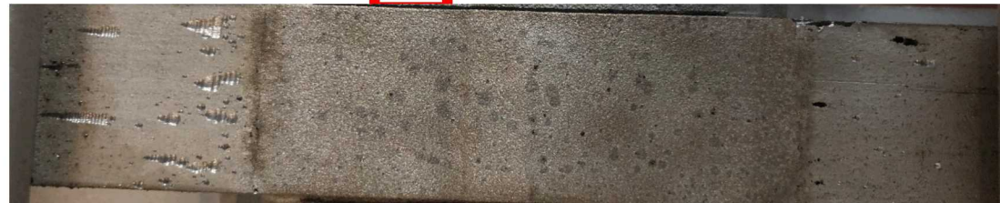
Inconel 625 sprayed coupon (No crack after 216h) (Delamination observed)
