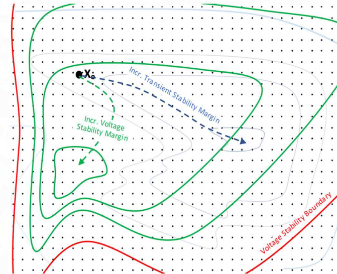
Transient & Voltage Stability Level Curves
