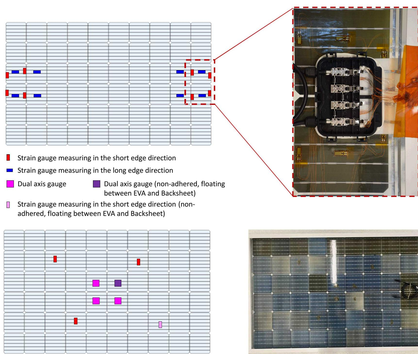
Modules have been received at Sandia with gauges mounted at locations of interest
