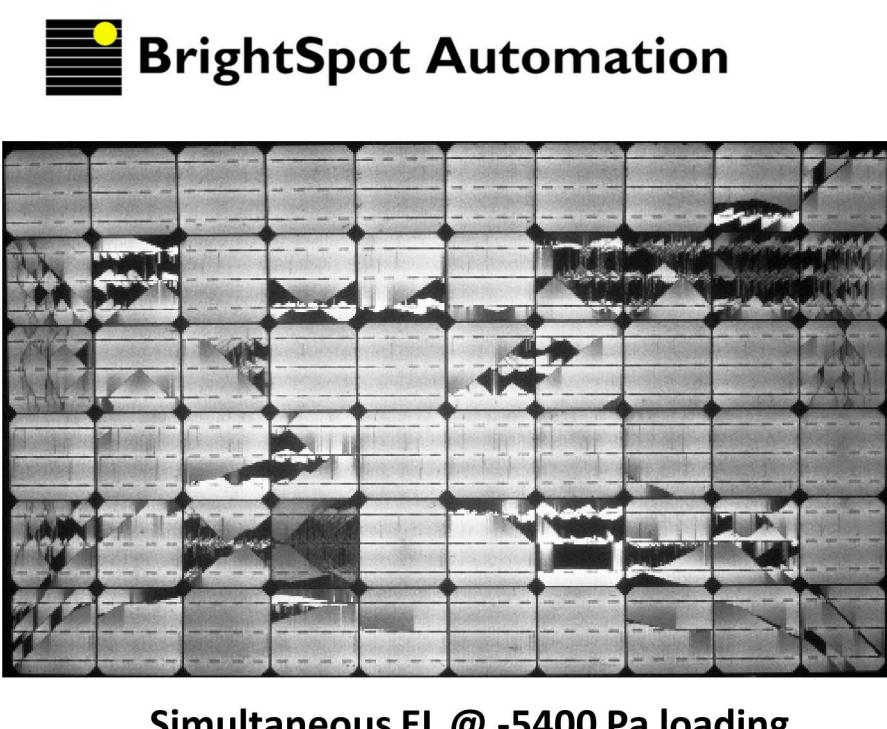
Load Spot mechanical tester enables controlled module loading with simultaneous internal & external measurements
