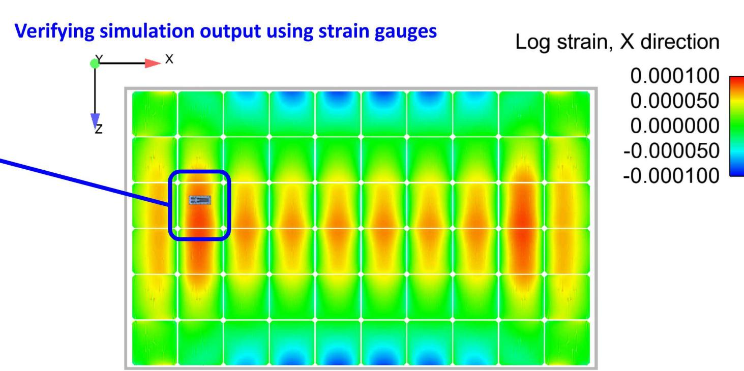
Can we verify that simulations predict the correct internal strain in a full PV module? Can gauges report fielded module strain?
