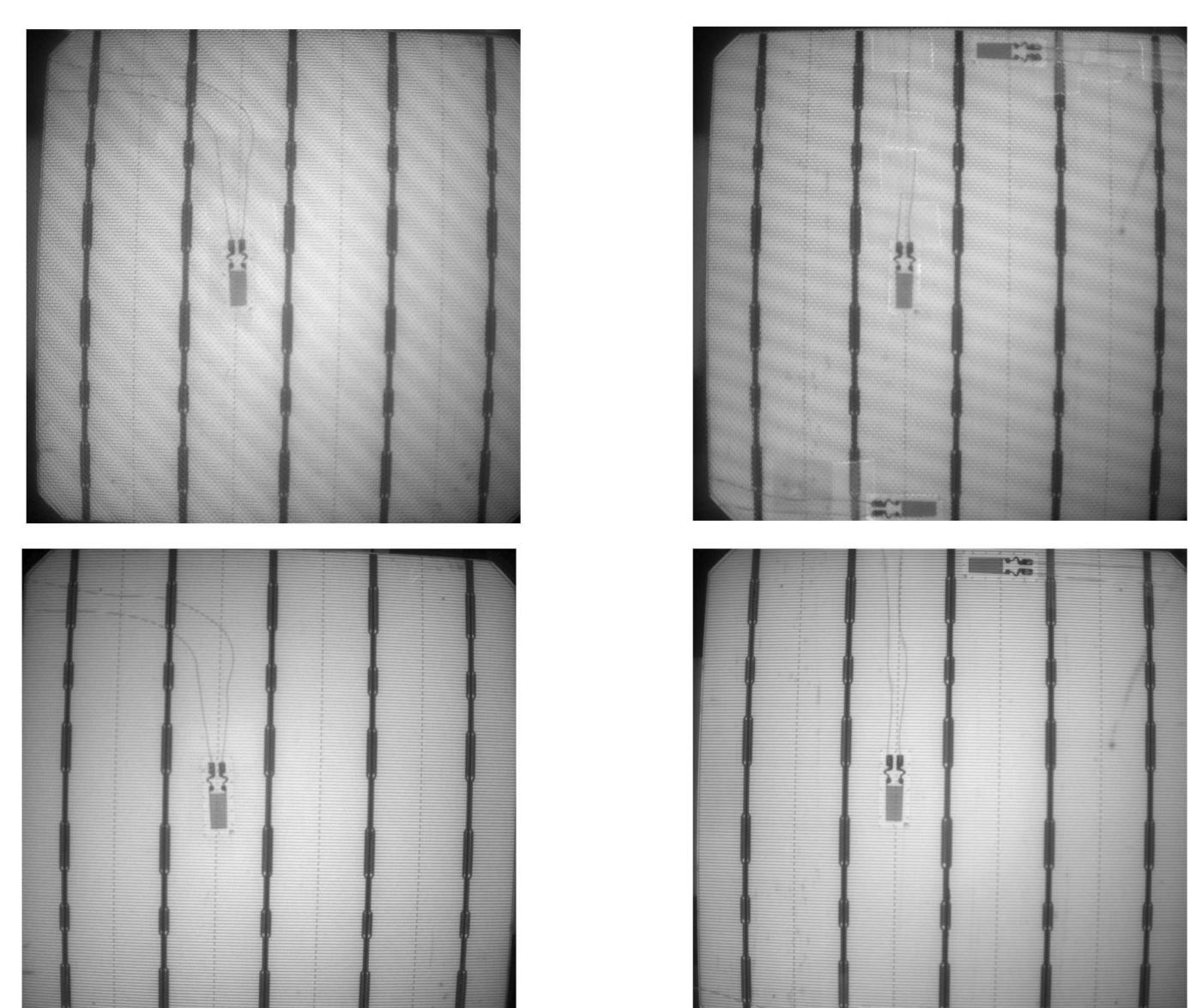
Photoluminescence images of two example gauge/wire placements
