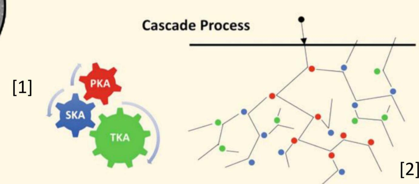
Ion and neutron particle bombardment can cause damage cascades in metals as well as transmutation reactions.
