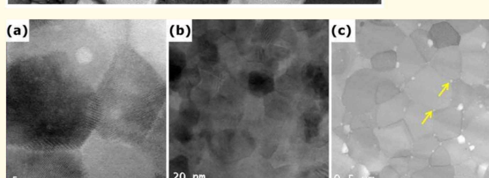
Smaller grains and twin boundaries should be more effective radiation defect sinks due to the increase in interfacial boundary area
