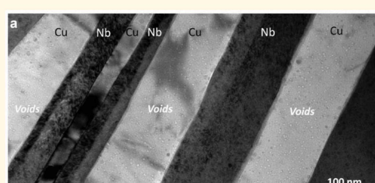
Interfaces have been shown to be effective sinks for collecting and annihilating radiation defects
