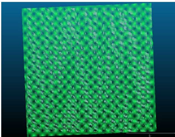
Figure 8. Facet point cloud and fitted plane. Figure 9. Facet points and plane from edge view
